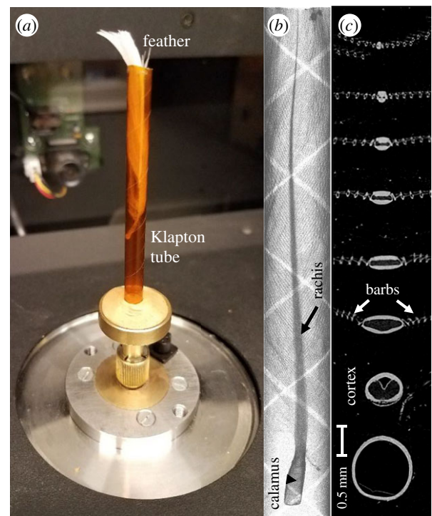
Figure 4. (a) Feather inside an X-ray invisible tube (Klaption) mounted in the \mu CT scanner. (b) \mu CT-scanned image of the feather. (c) Reconstructed images of feather cross section. The cortex of the rachis is the white, thin-walled structure region. Small white dots that eventually appear to the left and right of the rachis are the barbs and barbules, which are filtered out during image processing. (Online version in colour.)
